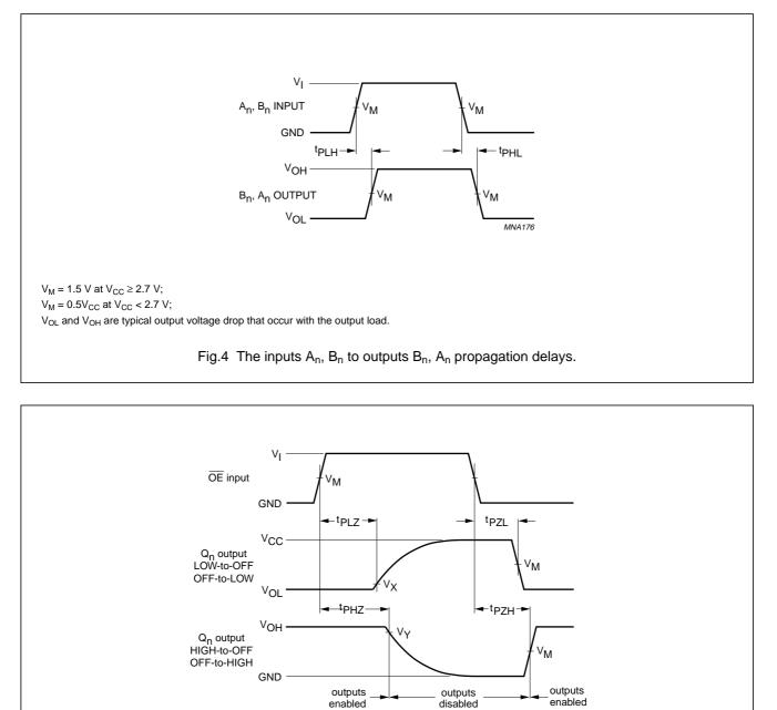
$$\begin{split} V_M &= 1.5 \ V \ at \ V_{CC} \ge 2.7 \ V; \\ V_M &= 0.5 V_{CC} \ at \ V_{CC} < 2.7 \ V; \\ V_X &= V_{OL} + 0.3 \ V \ at \ V_{CC} \ge 2.7 \ V; \\ V_X &= V_{OL} + 0.1 \ V \ at \ V_{CC} < 2.7 \ V; \\ V_Y &= V_{OH} - 0.3 \ V \ at \ V_{CC} \ge 2.7 \ V; \\ V_Y &= V_{OH} - 0.1 \ V \ at \ V_{CC} \ge 2.7 \ V; \\ V_Y &= V_{OH} - 0.1 \ V \ at \ V_{CC} \ge 2.7 \ V; \\ V_Y &= V_{OH} - 0.1 \ V \ at \ V_{CC} < 2.7 \ V. \end{split}$$
